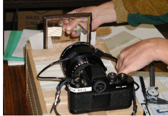
Fig. 1. Photographic set up for taking pictures of the foot. The bird's right foot was softly pressed against the glass while taking the pictures
